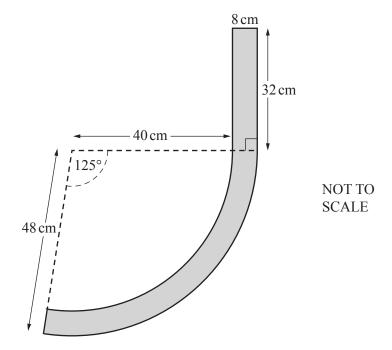
The diagram shows the cross section of part of a park bench. It is made from a rectangle of length 32 cm and width 8 cm and a curved section. The curved section is made from two concentric arcs with sector angle 125°. The inner arc has radius 40 cm and the outer arc has radius 48 cm.
